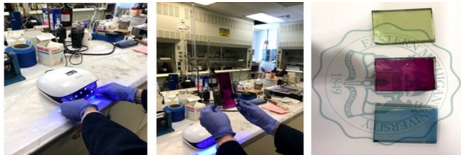
(c) Photochromic activity of coatings by light exposure.
