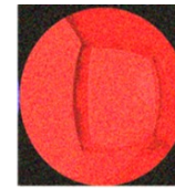
(a) Red photochromic glass with imperceptible glare (26% DGP).
