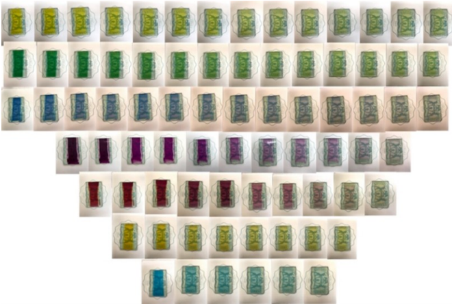
Figure 3. The developed photochromic coatings upon exposure to UV for a specific time.
